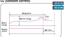
[Termination conditions] Time, voltage, -∆V, temperature, and  $\Delta T/\Delta t$
