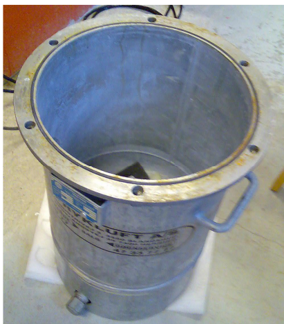
Figure 3: Example of a suitable steel container. The container needs to be decoupled properly from the floor and still be placed in a very quiet place this means no heavy traffic outside the building – no doors slamming – no people talking etc....
