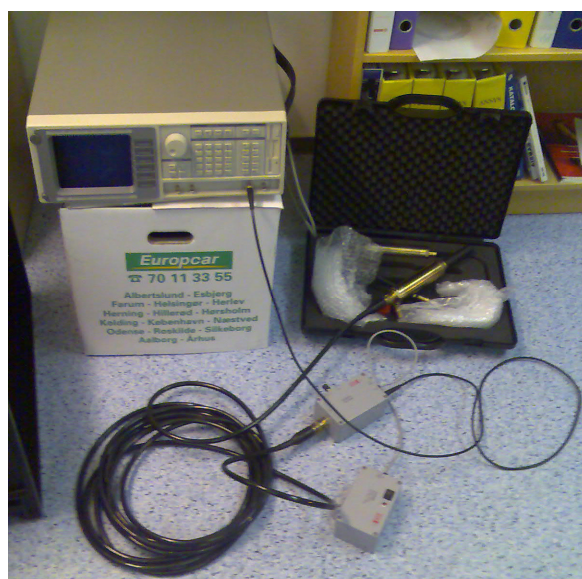
Figure 6: The open office setup – no shielding, 10meter cable between hydrophone and input module. A setup like that is simply not good enough for a proper own noise measurement.
